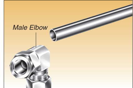
The male elbow is positioning in the wrong direction.
